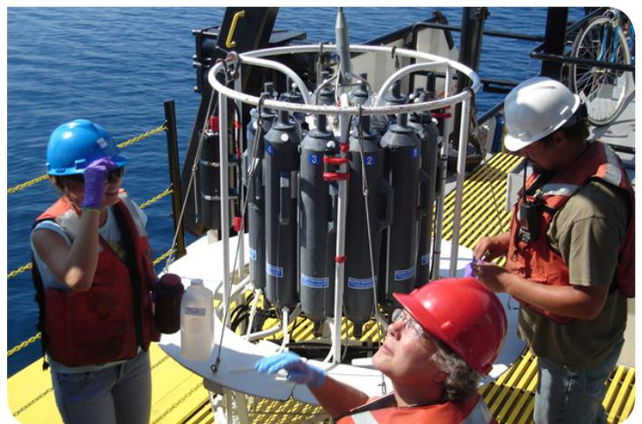
Sampling crews prepare to lower the sampling rosette to collect water samples using clean sampling techniques on Lake Erie.
